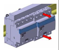
Pull the device downward in order to release it completely from the prongs of the busbar
