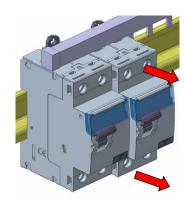
Pull the device downward in order to release it completely from the prongs of the busbar
