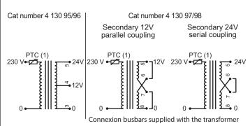
b. Bell transformer: safety isolating transformer with secondary voltage not permanently exceeding 24V and for a non permanent using.
