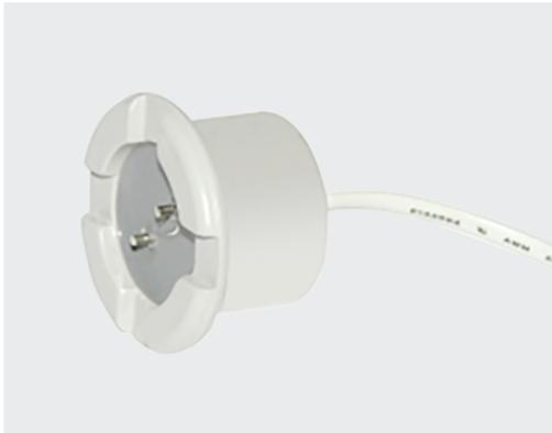
The water logging sensor can provide an output signal. When the water logging is high enough to reach at the sensor probes (about 1mm above the test surface), it sends an alarm signal.
