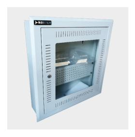
The Easycab range of recessed type wall mount cabinets designed for home/office environment. The cabinet's structure is welded and painted with electro static powder coated finish. Easycab is available in 12U size and comply with ANSI/EIA RS-310-D. DIN41497 part 1, IEC 297-2, DIN41497 part 7, GB/T3047, 2-92 standards.
