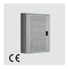
The Smart cab range of Flush-Mount type wall mount cabinets designed for home/office environments. The cabinet's structure is welded and painted with electro-static powder coated finish and will comply with ANSI/EIA RS-310-D, DIN41497 part 1, IEC 297-2, DIN41497 part 7, GB/T3047, 2-92 standards.
